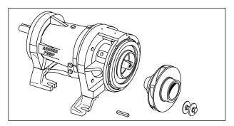
C. Impeller and Key Removed.
